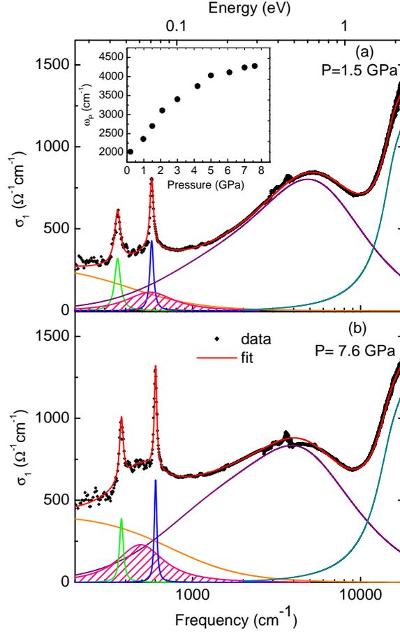
**Figure 3.** Fit of the RT optical conductivity  $\sigma_1$  at (a) 1.5 and (b) 7.6 GPa using the Drude-Lorentz model. The far-infrared band is highlighted by hatching. Inset: Plasma frequency  $\omega_P$  of the Drude term as a function of pressure obtained from the Drude-Lorentz fitting.
