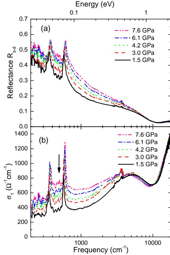
**Figure 2.** (a) Pressure-dependent reflectance at RT and (b) pressure-dependent real part of the optical conductivity at RT obtained by KK analysis. The arrow in (b) marks the far-infrared band as discussed in the text. The small features at around  $3600 \text{ cm}^{-1}$  are artifacts due to multi-phonon absorptions in the diamond anvil.
