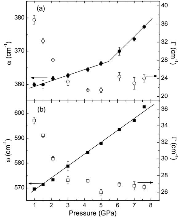
**Figure 6.** Phonon frequencies and linewidths as a function of pressure obtained by Drude-Lorentz fitting of the optical conductivity spectra. The lines are linear fits to the data points, in order to obtain the linear pressure coefficients.
