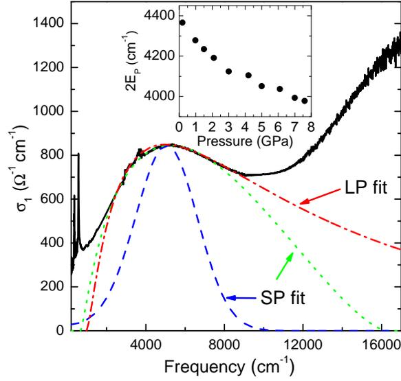
**Figure 7.** Comparison between the fitting curves of the experimental optical conductivity data at 1.5 GPa using the LP model [Eq. (2), dashed-dotted line], the SP model in the limit  $s \gg D$  [Eq. (4), dashed line], and the SP model in the limit  $s \ll D$  [Eq. (5), dotted line]. The inset displays the parameter  $2E_P$  as a function of pressure, obtained from the fitting using Eq. (5).
