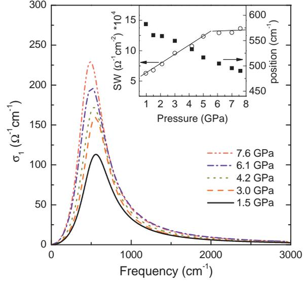
**Figure 5.** Far-infrared band for selected pressures, obtained by Drude-Lorentz fitting of the optical conductivity spectra. Inset: Position and spectral weight of the far-infrared band as a function of pressure. Lines are guides to the eye.
