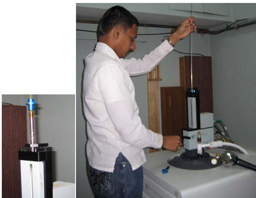
Figure 4: Mr Iyer loading the Mcell Ultra in a MPMS-XL7.
