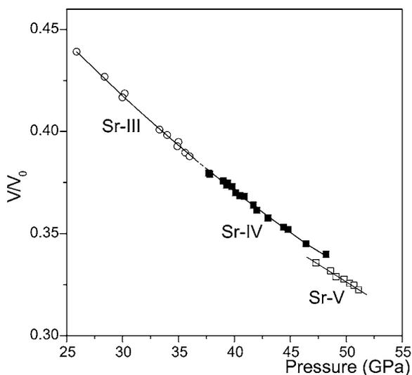
FIG. 5.  $V/V_0$  for Sr-III, Sr-IV, and Sr-V, where  $V$  is the atomic volume and  $V_0$  is its value in Sr-I at ambient pressure. The lines through the data are guides for the eye. No data points are plotted between 36.0 and 37.7 GPa, the range where there are additional unexplained peaks (see text).
