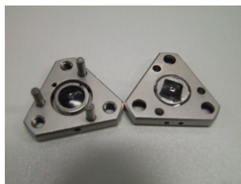
Figure: M-A-II with reglued anvils
